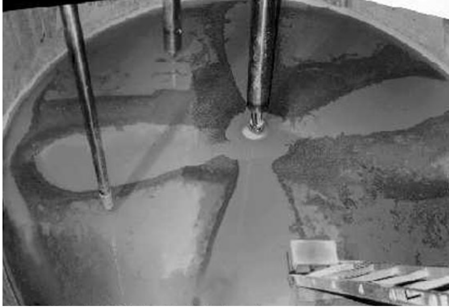
Fig. 2. Russian Pulsating Mixer Pump-Cleaning footprint of initial test at PNNL's quarter-scale test facility.
