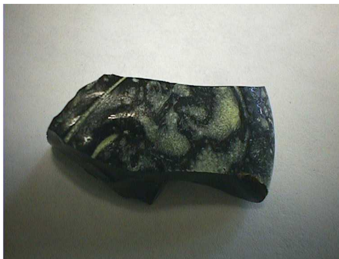
Fig. 3. Visible Salt Segregation
