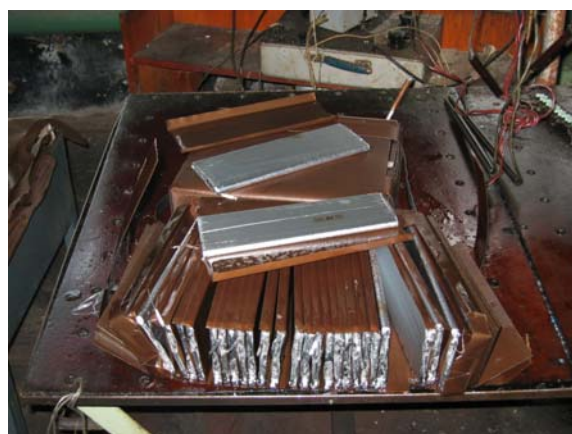
b) Typical internal capacitor contents
