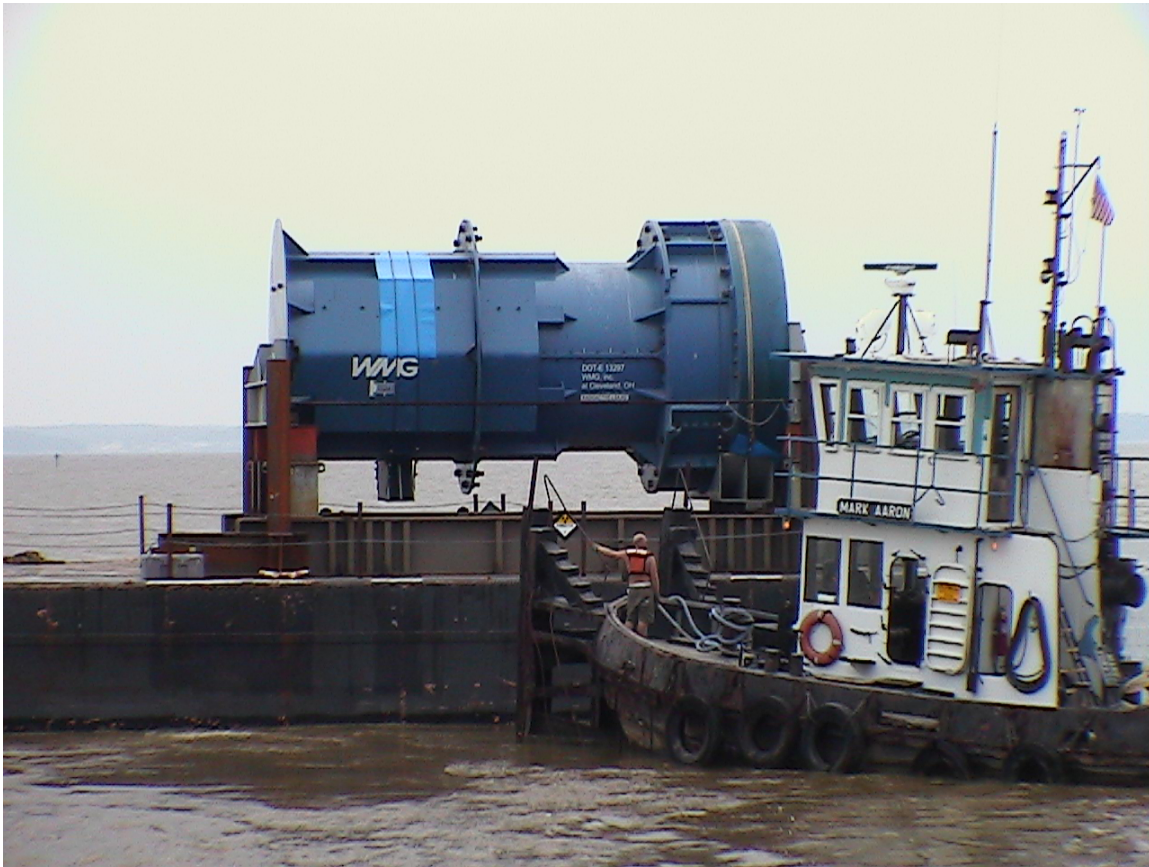
Fig. 3. Surry unit 2 RPV head package on barge
