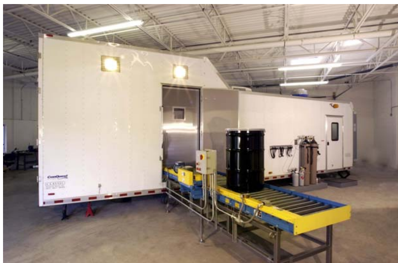
Fig. 1. Mobile Drum Venting System
