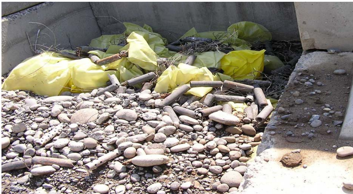
Fig. 4. Material Suspected of Containing Highly Radioactive Fuel Elements Fragments.
