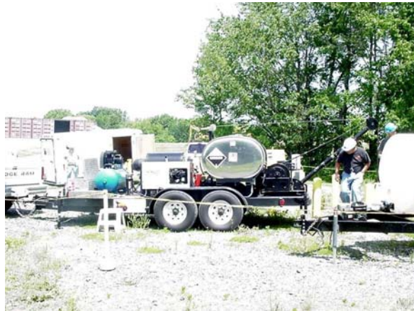
Fig. 1. MW rehabilitation "Stinger" rig
