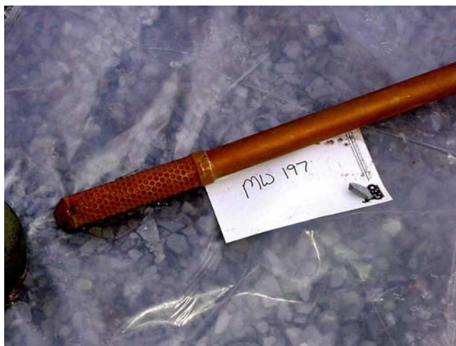
Fig. 3. MW197 pipe and screen
