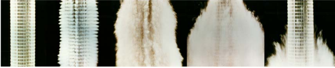
Fig. 3. Moving across the photograph from left to right: the metal fibre element loaded with dust; the dust is removed from the surface by the pulsed jet action; the dust is carried away; the dust begins to settle; and quickly falls to the bottom of the vessel leaving a clean element. Sequence time – less than half a second. The cleaning pulse is made whilst process flow continues.
