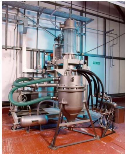
Fig. 4. MOX pellet grinding pulsed jet filter Installed in MFX test and development Facility
