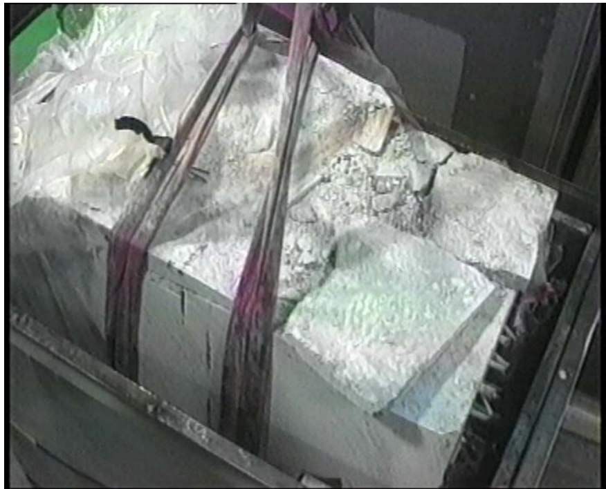
Fig. 2. Unloading of the concrete block from the shielding box
