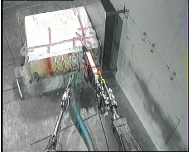
Fig. 1a. Coupling system, percussion jackhammer and suction hose of the vacuum cleaner
