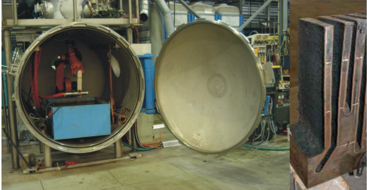
Fig. 2. Left: Test rig (pressure tank) at the Underwater Technology Center, Hanover. Right: Cutting edge of the mock up 70 – 130 mm; 5 th section of the thermal shield, plasma gas: Ar/H 2 , secondary gas: air, cutting current: 900 A, cutting voltage: 215 – 220 V, cutting speed: 240 mm/min (70 mm) – 90 mm/min (130 mm), cutting position: vertically descending – horizontal.
