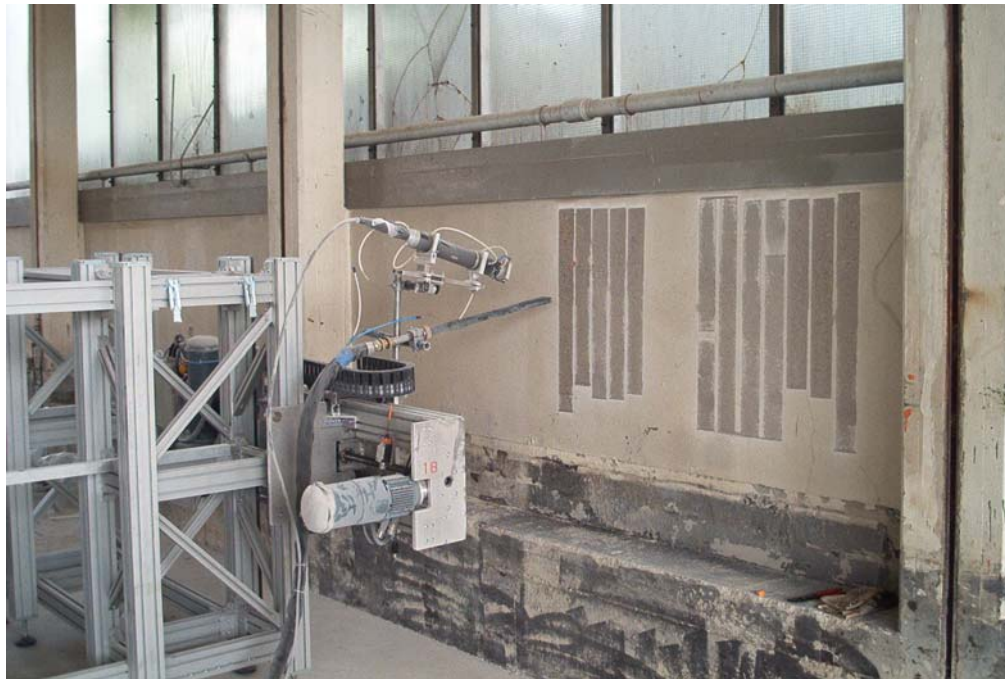
Fig. 1. Test of the dry ice laser beam process at the Forschungszentrum Karlsruhe
