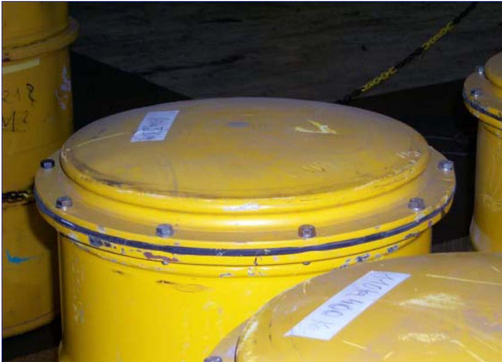
Fig. 1. Pressure build-up in a waste drum
