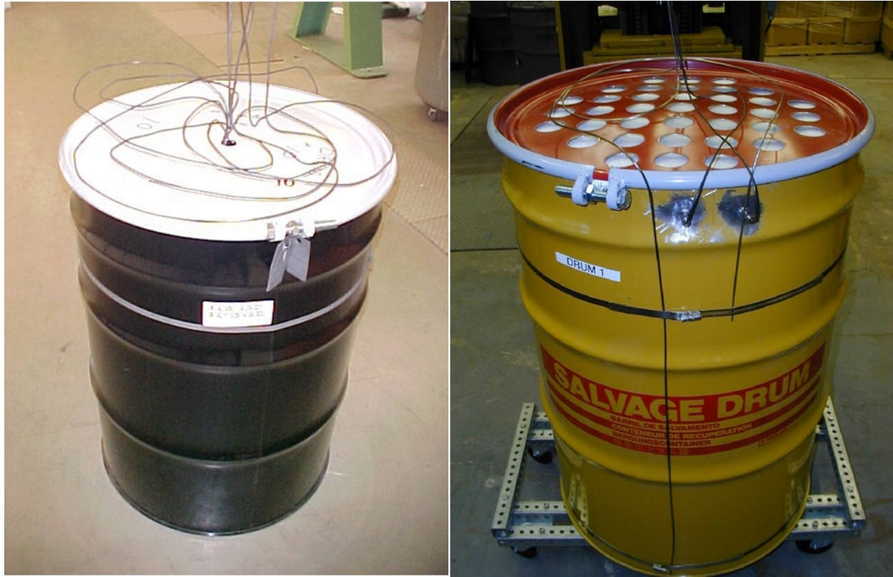
Fig. 2. Assembled 55-gal. drum (left) and assembled 85-gal. overpack containing a 55-gal. drum (right)
