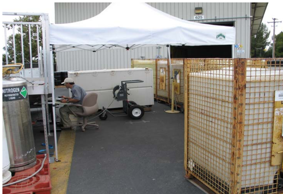
Fig. 3. MCS Technical Supervisor Richard Machado analyzing waste box using tandem ISOCS units, Lawrence Livermore National Laboratory, Livermore California.
