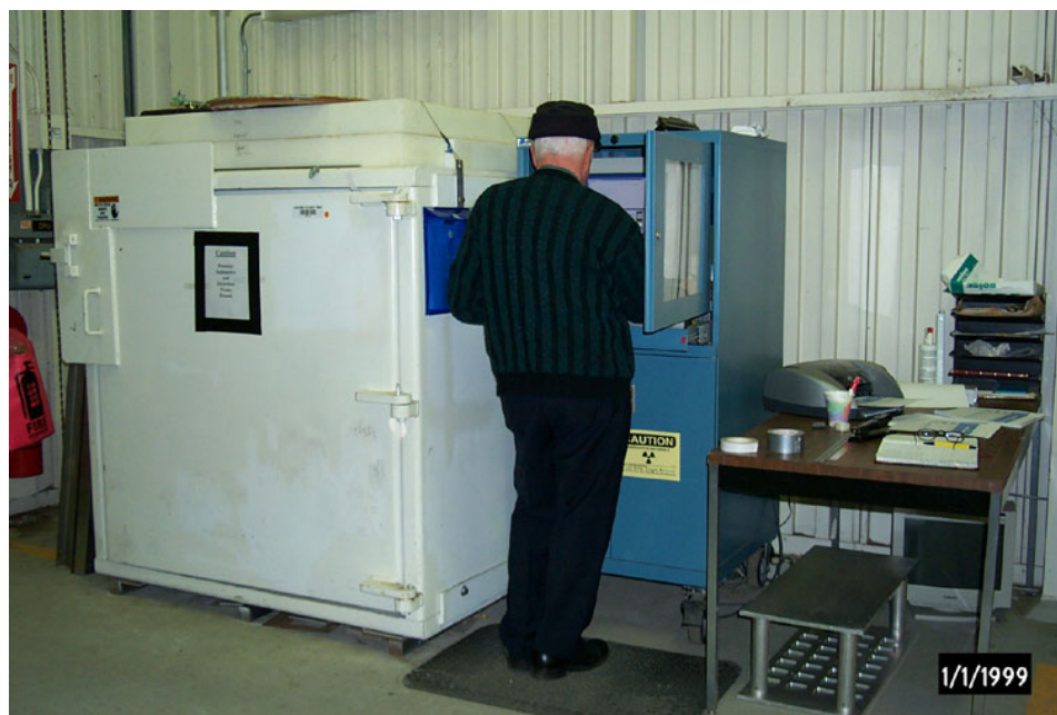
Fig. 2. Dale Hankins completing start-up of the RHWM NDA Unit, a shielded gamma and passive neutron assay unit, Lawrence Livermore National Laboratory, Livermore California.
