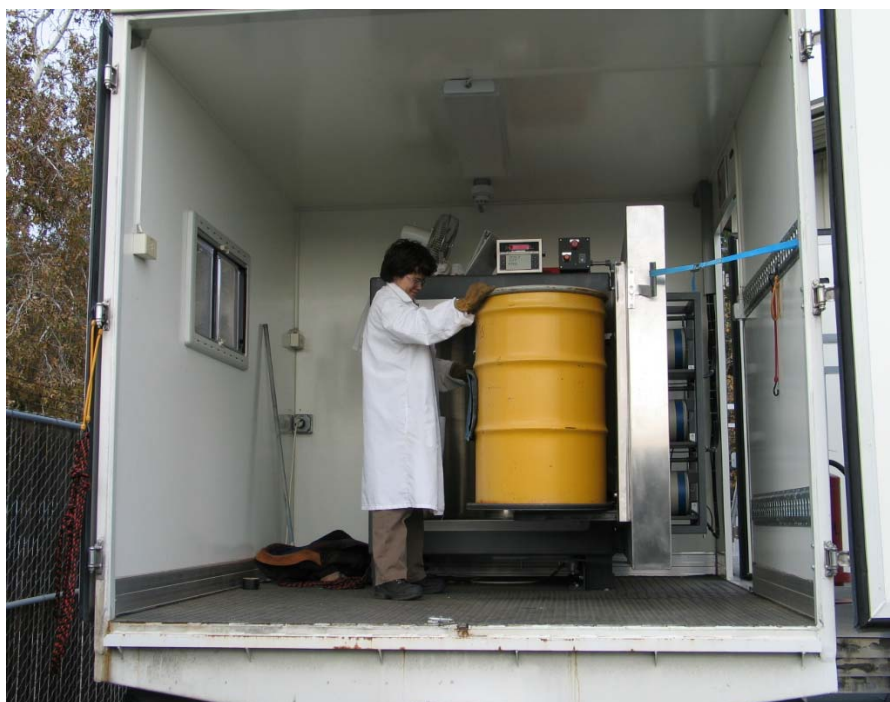
Fig. 4. MCS assay operator Tracy Jue securing drum to Q2 waste assay system turntable, Lawrence Livermore National Laboratory, Livermore California.
