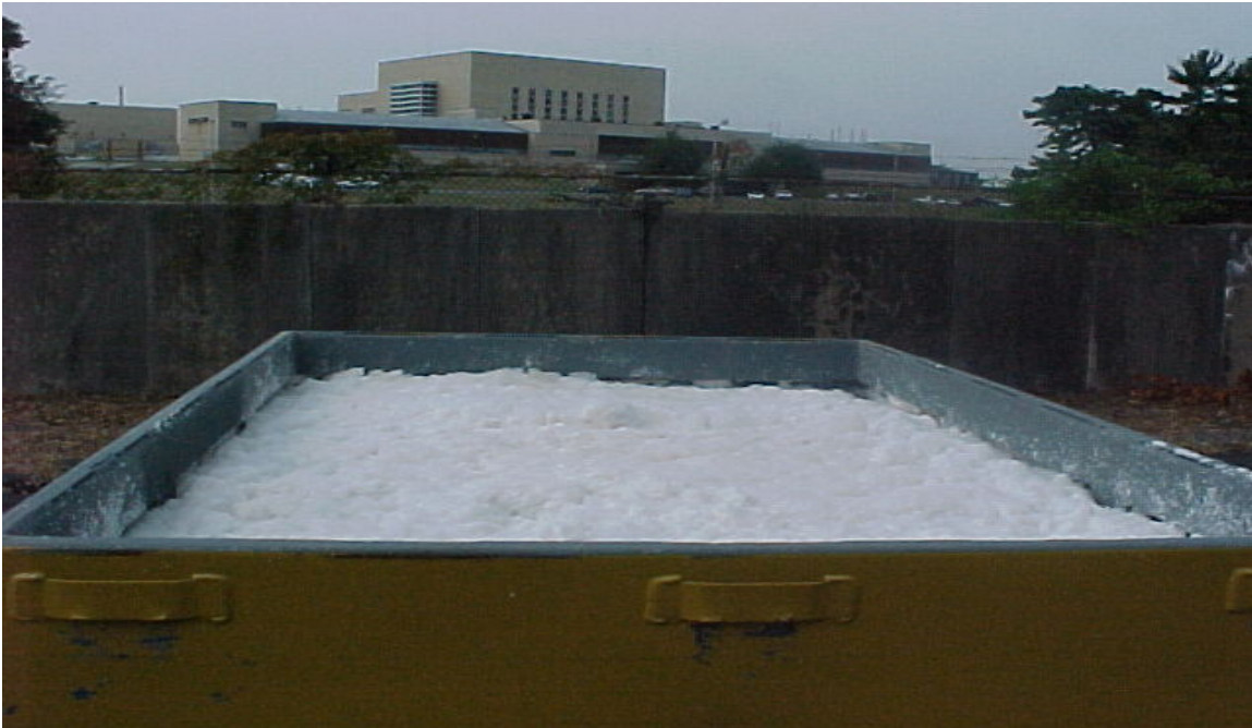
Fig. 2. Solidified LLLRW after Shake Test
