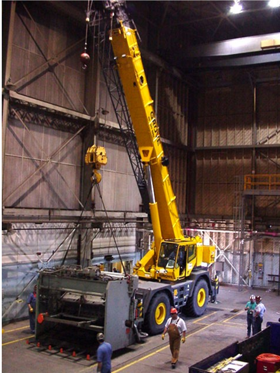
Fig. 1. Typical Equipment Move – 40,000 kg (44 ton) Shear Being “Walked” out of Shop
