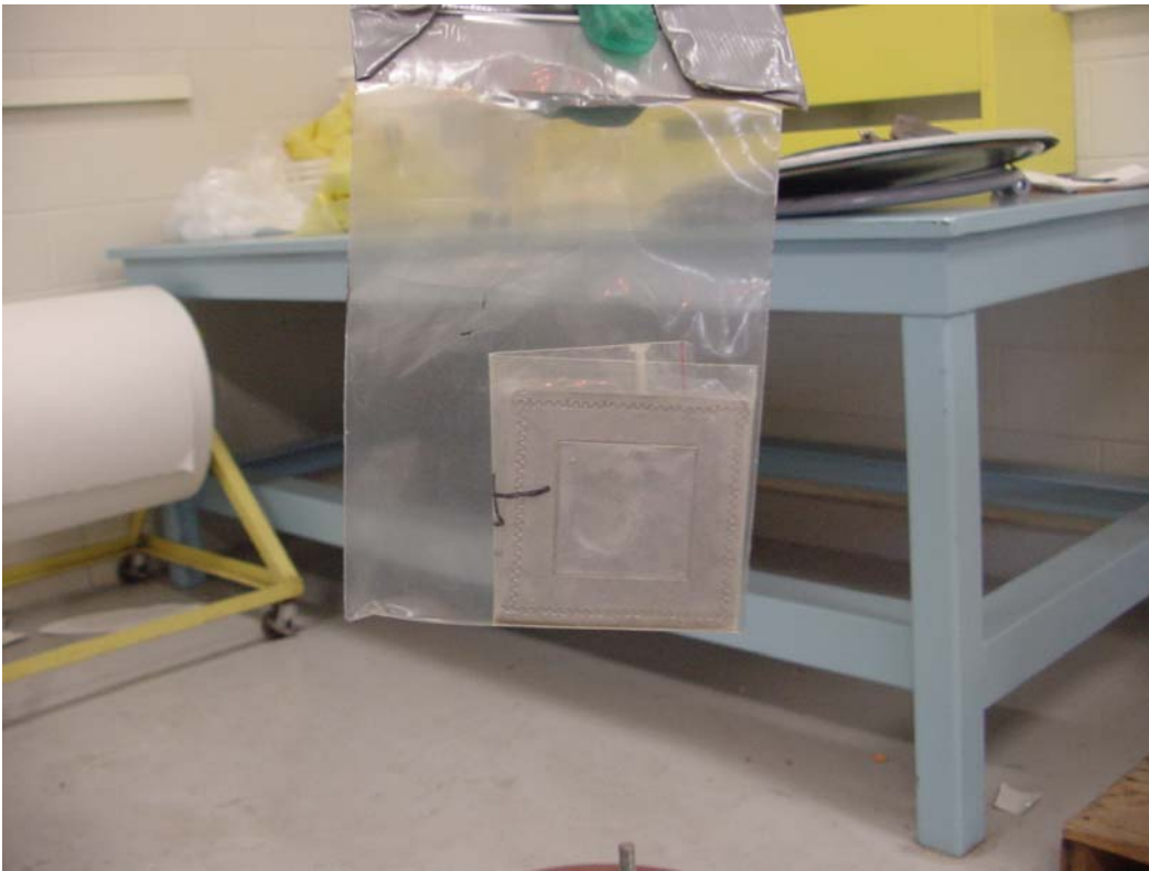
Fig. 3. Plutonium-239 foil removed from the steel holders and individually wrapped in a plastic bag.
