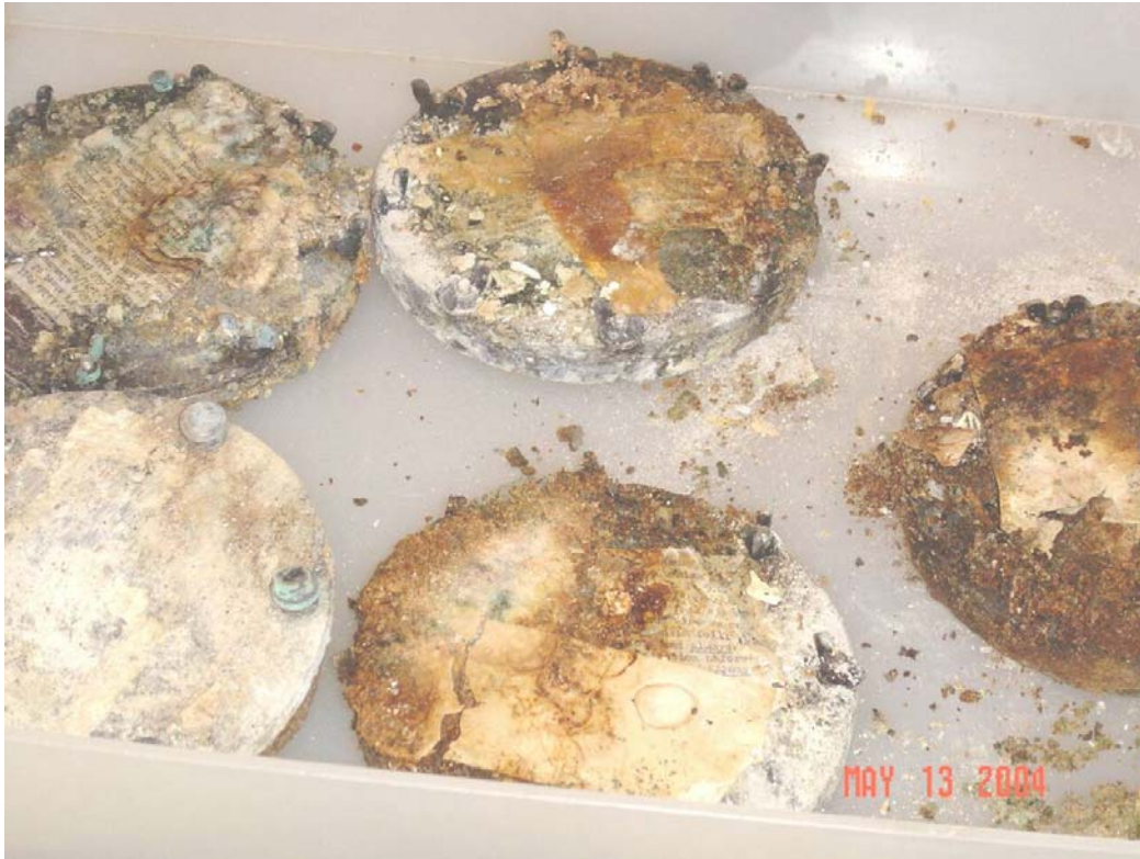
Fig. 2. Plutonium foils inside of aluminum holders.
