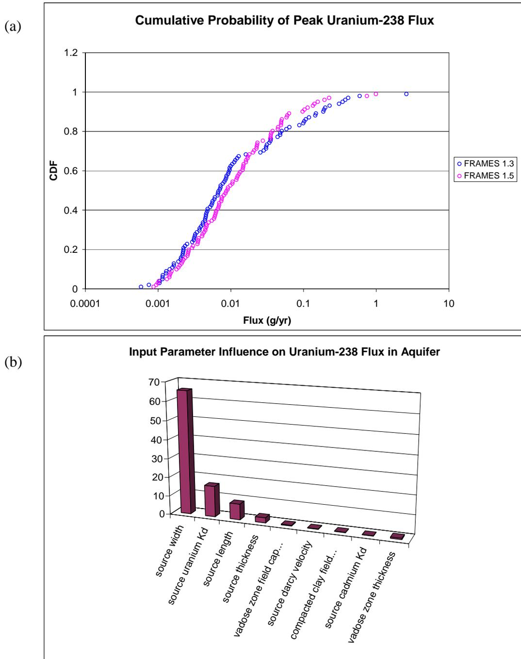
**Fig. 3. (a) Comparison of CDFs for uranium-238 flux in the aquifer using FRAMES 1.3 and FRAMES 1.5. (b) Input parameter importance on flux of uranium-238 in the aquifer using both present-day and future conditions. Flux was recorded approximately 115 meters below the source zone.**
