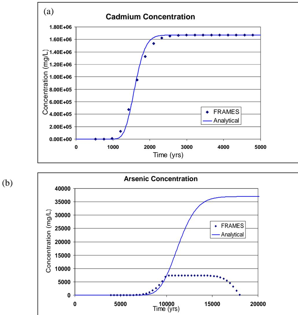
**Fig. 1. (a.) Deterministic results for cadmium concentration as a function of time. (b) Deterministic results for arsenic as a function of time; the FRAMES concentration curve plateaus at 10,000 years as a result of a bug in the software. The concentrations are recorded at the exit of the vadose zone ( $x=6$  m).**
