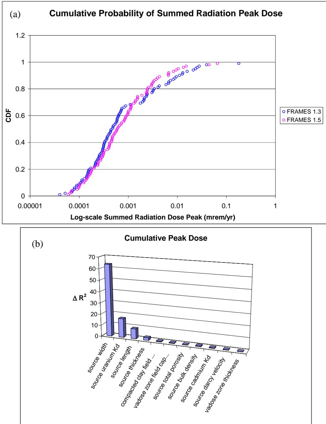
**Fig. 4. (a) Comparison of FRAMES 1.5 and FRAMES 1.3 summed radiation dose. (b) Input parameter influence on summed radiation dose for present-day conditions. Peak dose was recorded approximately 115 meters below the source zone.**
