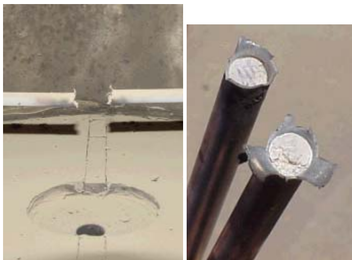
Fig. 2. Disrupted CeO2 test rodlet
