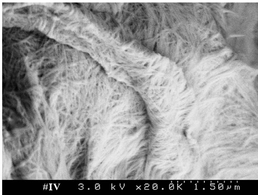
Fig. 1. SEM photograph of the sludge like solid form in the reaction of phosphoric-hydrochloric acid with uranium metal
