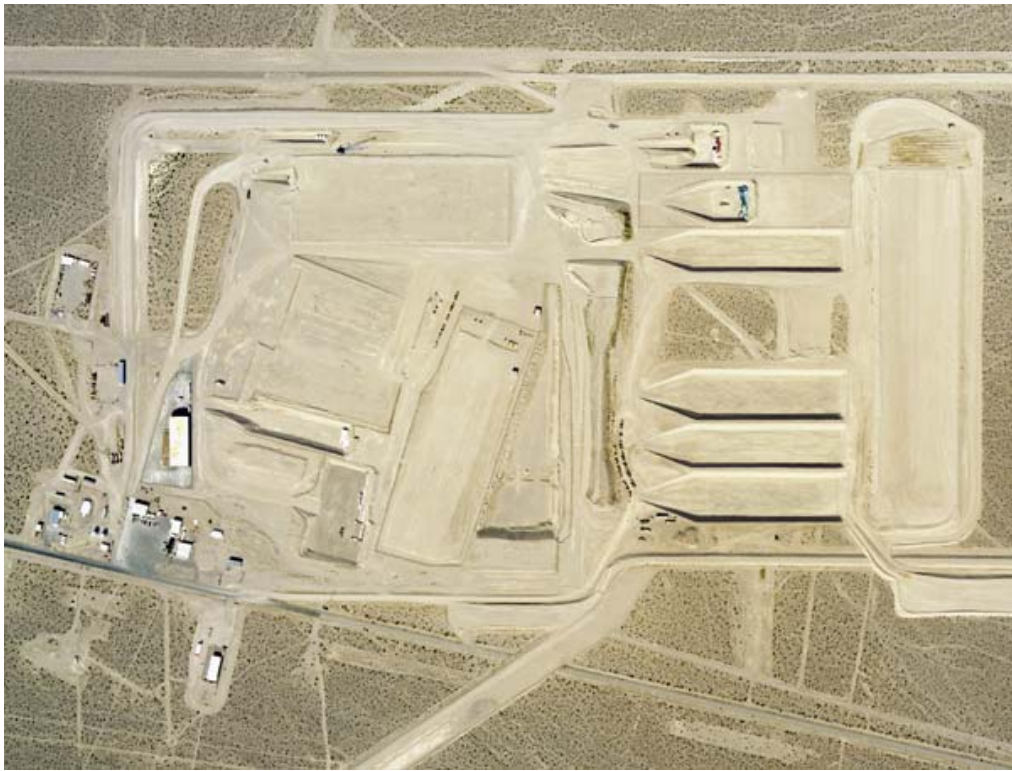
Fig. 1. Color aerial photograph of the Area 5 Radioactive Waste Management Site (RWMS). Low-level and minor volumes of mixed radioactive waste are disposed in shallow trenches, pits and large diameter boreholes. Inactive waste cells are covered with an operational cover of alluvial soil. The support facilities for the RWMS are in the lower-left corner of the photograph.
