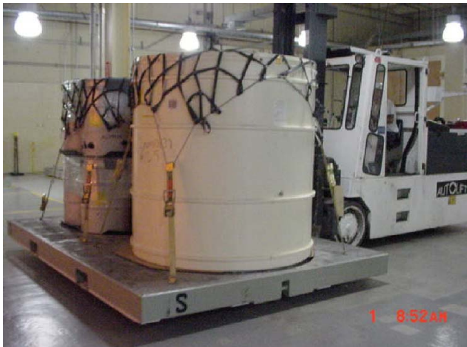
Fig. 2. TRU waste (in TRU-PAC containers) being unloaded at the WIPP facility.
