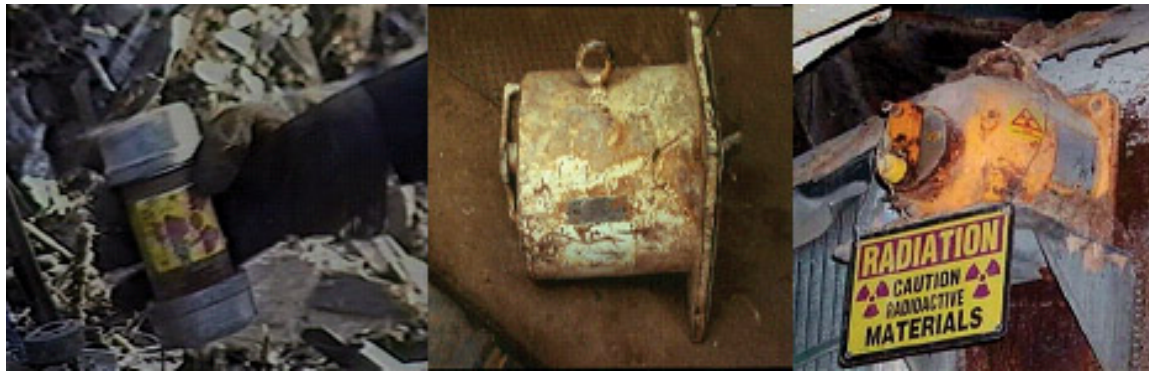
Fig. 2. Examples of radioactive sources from demolition sites.
