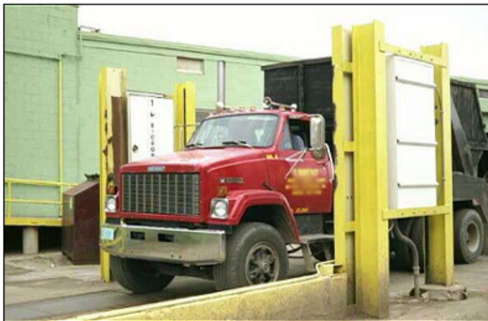
Fig. 1. Radiation Portal Monitor at entrance to scrap yard.
