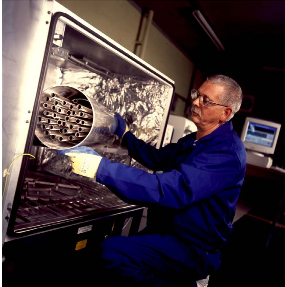
Fig. 4. Measurement chamber being loaded with a batch of AGR fuel cans
