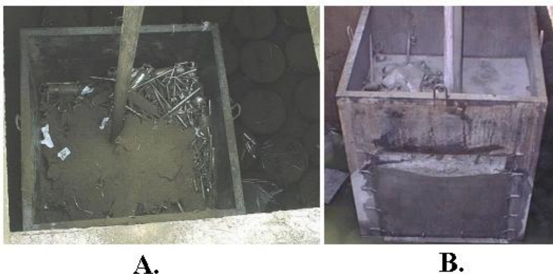
Fig. 3. Cementation by a impregnation method of mixing SRW in 4 m 3 container: A - SRW in 4 m 3 container; B - final product.
