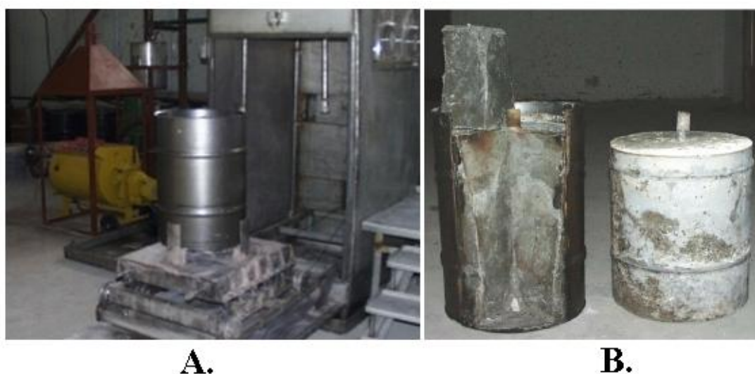
Fig. 2. Cementation by an impregnation method of ash residue in 200 l a barrel: A - trial installation; B – final product.
