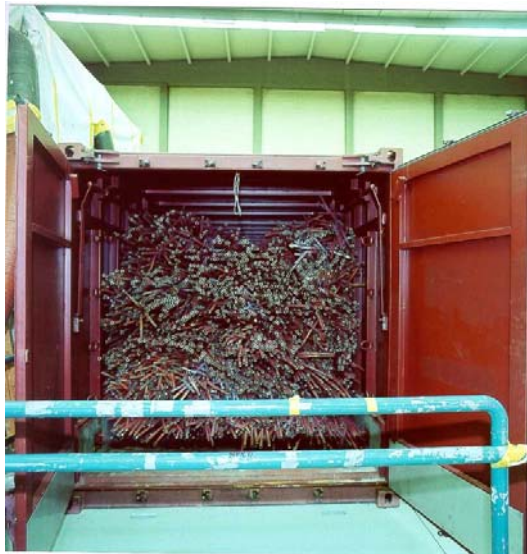
Fig. 2. 20'-Container with Condenser Tubes
