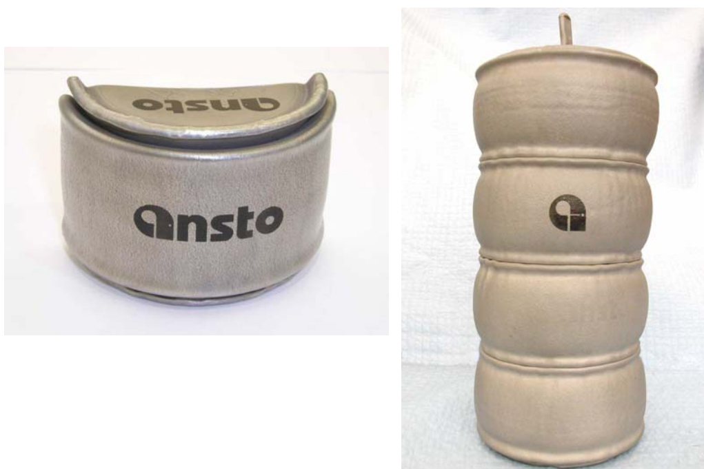
Fig. 3. Hot-isostatically pressed dumbbell-type cans used for Pu-doping work. The can on the left is the can that contains ~ 370 g of zirconolite-rich synroc containing ~ 50 g of PuO 2 and 18 wt% Gd, Sm and Hf neutron absorbers. The can is ~ 6 cm diameter by 4 cm high. The can on the right is a non-radioactive 5 kg scale up ~ 9 cm diameter by 18 cm high. The final size can be tailored by adjusting the starting geometry of the cans. Dumbbell-type cans containing up to 105 kg of waste form ceramic have been made.
