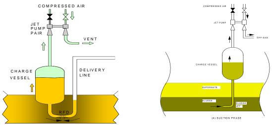
Fig. 1. A simplified fluidic pumping and mixing arrangement
