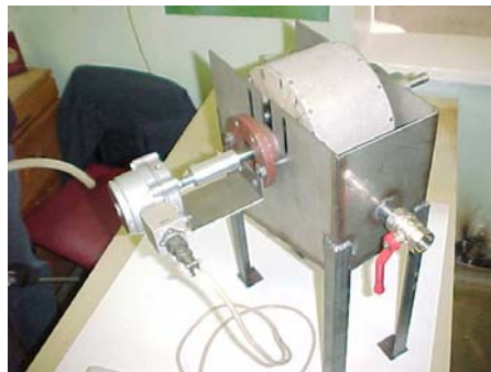
Fig. 4. Overview of laboratory drum-type vacuum filter
