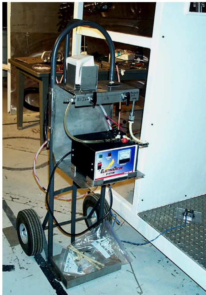
Fig. 3. ED Control Unit Modified for Remote Use.
