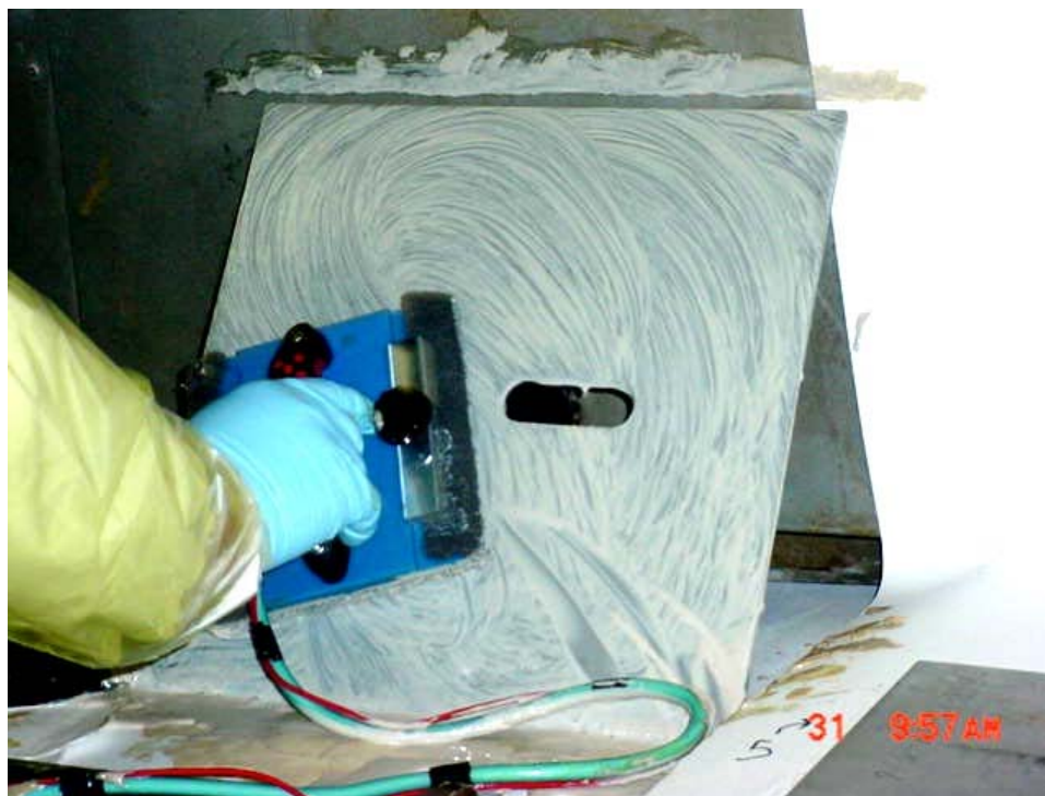
Fig. 4. ADA Technologies ElectroDecon System Being Used to Clean Criticality Barrier.
