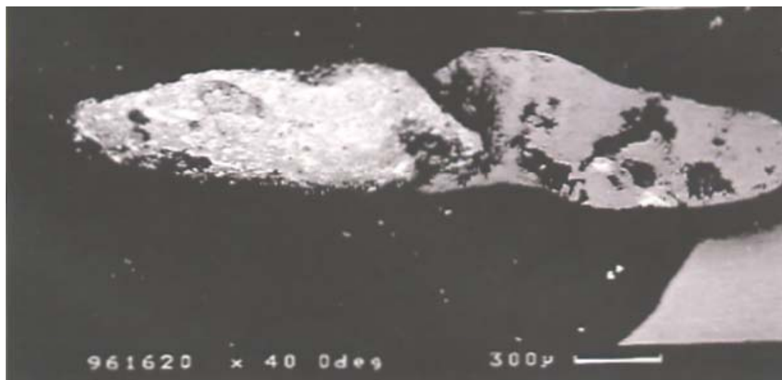
Fig. 1. Back-scattered electron image of a foreshore particle, whose weight is 1.25 mg, length is 2.5mm and maximum width is 0.5 mm, ^{137}\text{Cs} radioactivity is 1.6 \cdot 10^6 Becquerel per sample. The white spots show the distribution of uranium on the particle.
