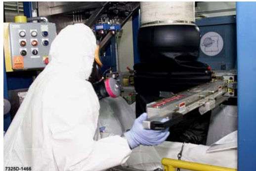
Fig. 3. Operator positions RF seal arm into position for liner closure.
