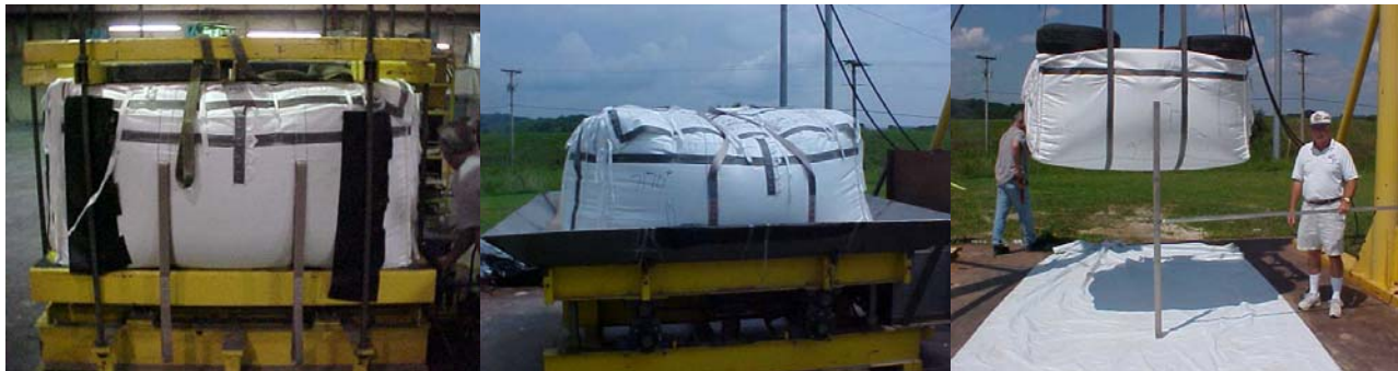
Fig. 8. The 24 - Hour stacking test with 5 times the package weight; The 2 - Hour vibration; The 4 - Foot drop test.
