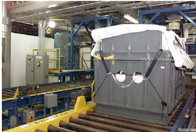
Fig. 2. The Lift-liner system in the loading frame is power conveyed to the load position.
