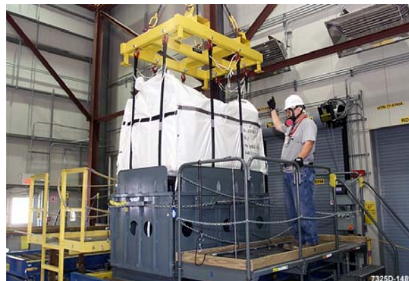
Fig. 5. The Lift-liner system is lifted out of load frame to be closed and prepared for shipment.
