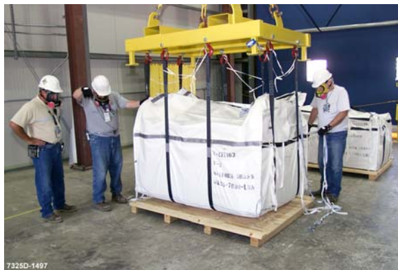
Fig. 7. Filled Lift liner package ready for shipment.
