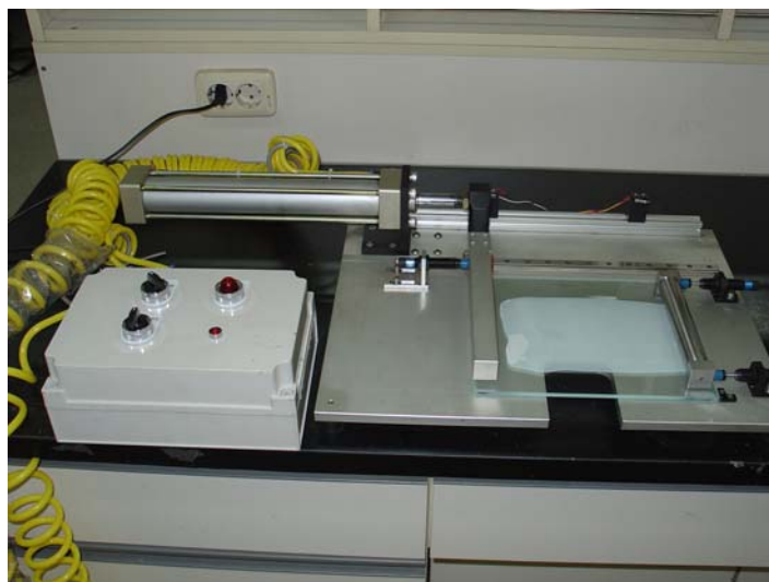
Fig. 1. Automatic casting machine for the polymer membrane preparation
