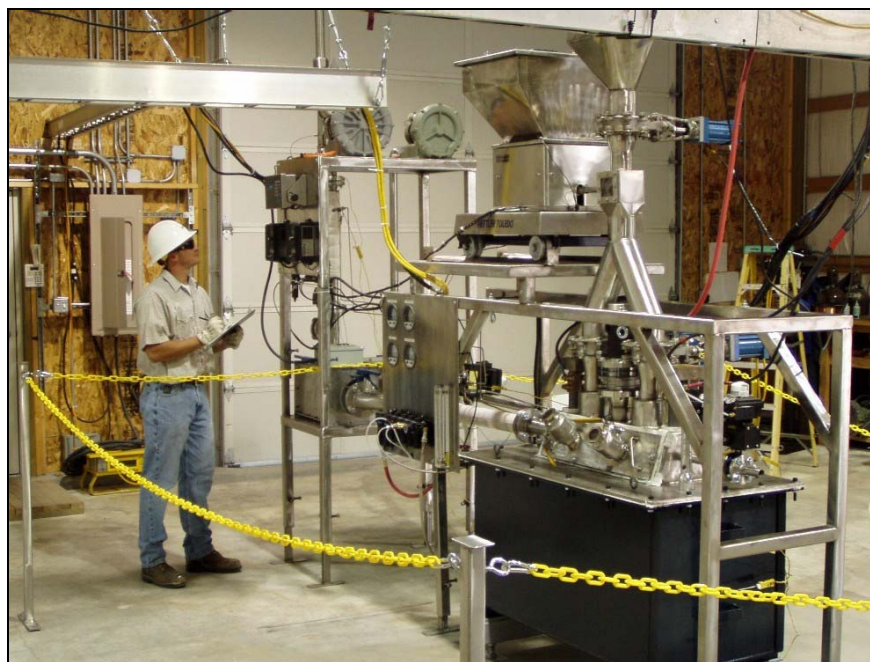
Fig 5. Photograph of 1/6 th scale bulk vitrification equipment.
