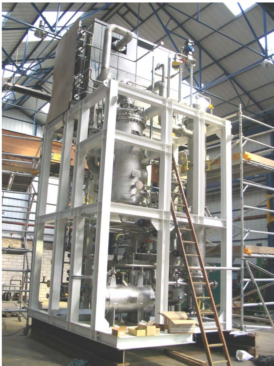
Fig. 2. One of the Evaporator Modules in Construction at Works
