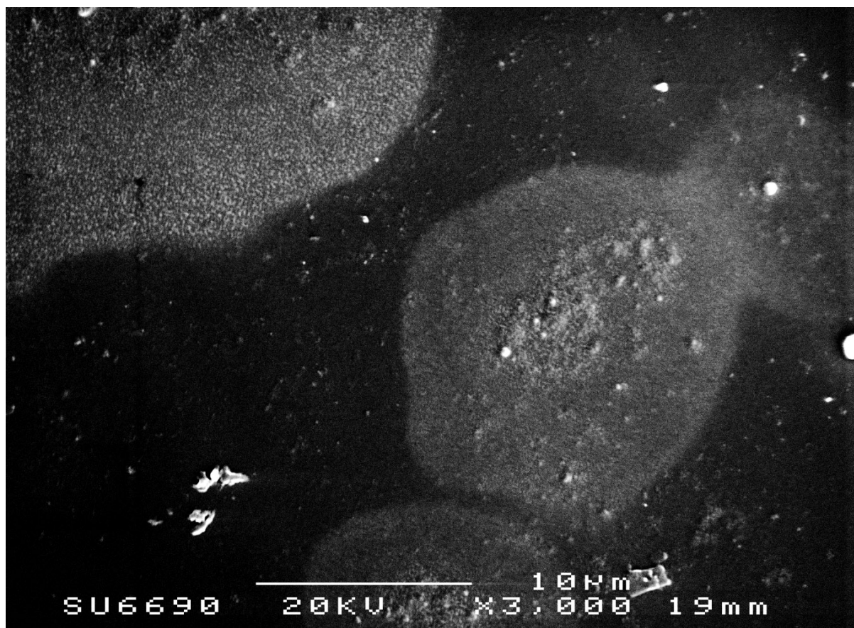
Fig. 2. British Magnox-waste glass secondary electron image.
