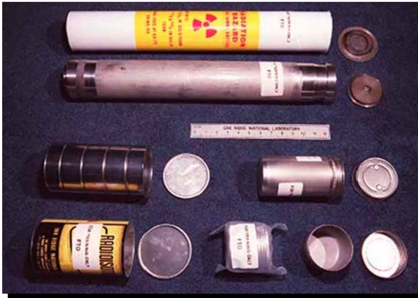
Fig. 6. Representative Outer Container Types Stored in Building 3019A Tube Vaults
