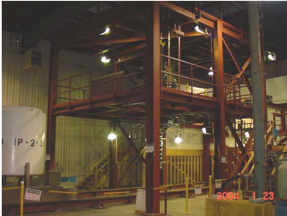
Fig. 1. The ITP prototype equipment included a container transfer car, gantry manipulator tool for remote closure with a riveting system, and product fill chute.
