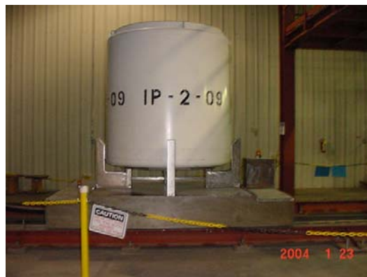
Fig. 2. Each IP-2 container can hold 160 cubic feet of liquid slurry mixed with solidification media is shown atop the transfer cart.
