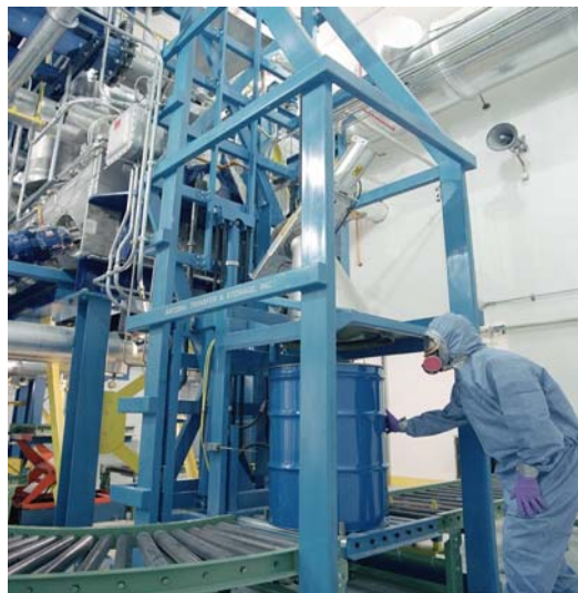
Fig. 2. Photograph of vertical lift and feed hopper mechanism.
