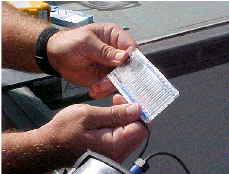
Fig. 5. Monitoring “chips” for measuring specific contaminants.
