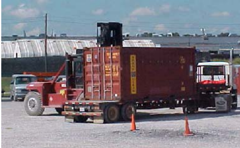
Fig. 1. A typical open-top container designed and constructed to represent a large, flat-bottom box with three walls, a door, and no ceiling. The dimensions are approximately 6.1 m (20 feet) in length, 2.4 m (8 feet) in width, and 2.6 m (8.5 feet) in height.
