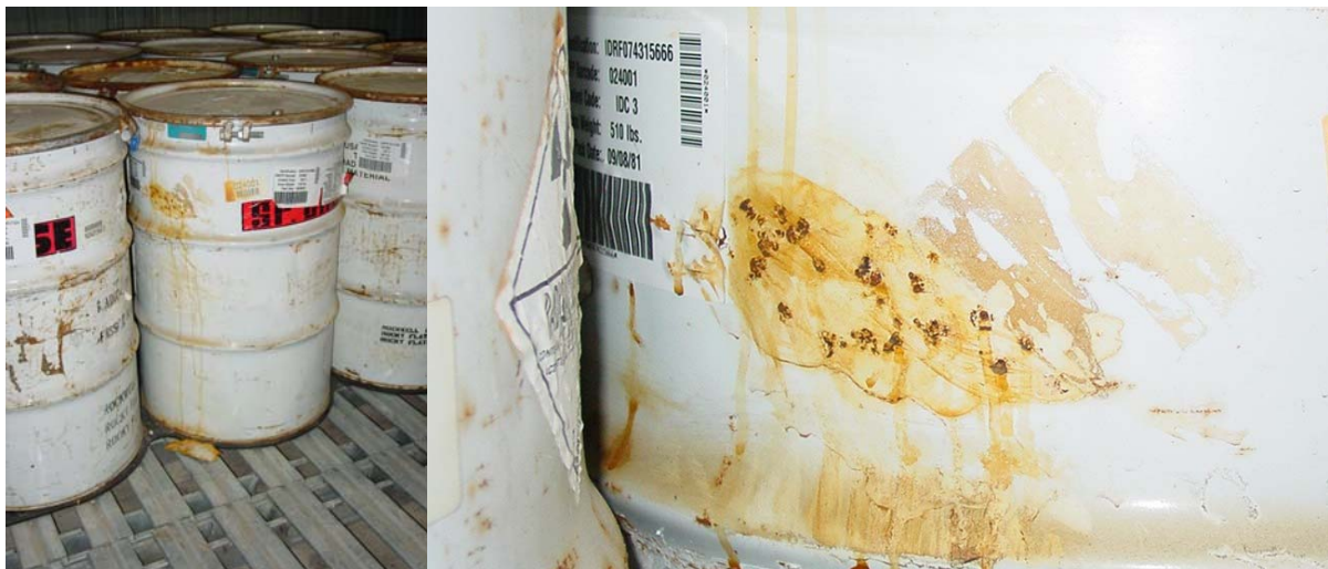
Fig. 4. Internal, Through-Wall Pitting
