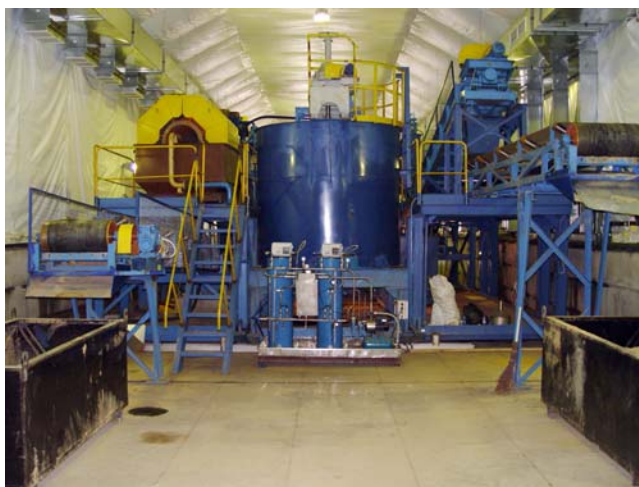
Fig. 4. Appearance of the pilot facility for wet decontamination of radioactively contaminated soil
