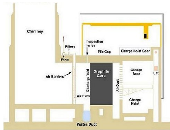
Fig. 1. Cross-section through Pile 1 structure a . Fig. 2. Graphite block arrangement in Pile 1 b
