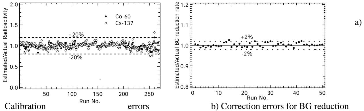
Fig. 4 Accuracies of calibration and correction for background reduction.
