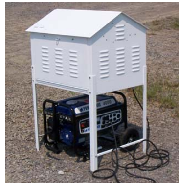
Demolition Boundary Air Monitors
