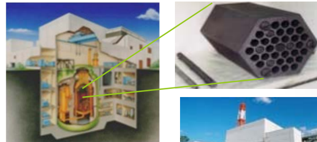
Fuel element for the HTTR - INL and JAEA collaborating to develop validated models for high temperature reactors
