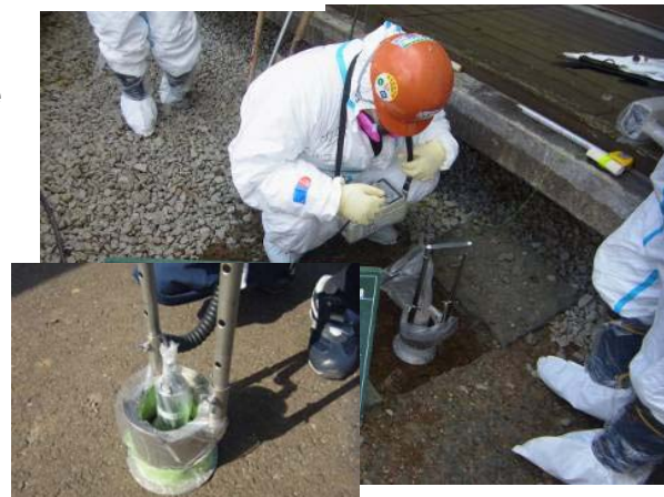
Measurement using the Collimator to eliminate scatter radiation from far area
