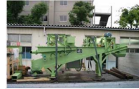
Wet sieving (particle-size Separation)
