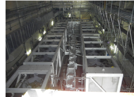
Plug-n-Process Modular Skid-Based System Allowed Fast Fabrication and Startup
