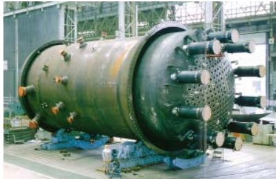
Reactor Pressure Vessel (RPV)
