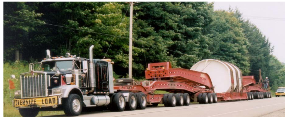
Transport CFMT Shipping Container from Fabrication Facility to On-Site Storage
