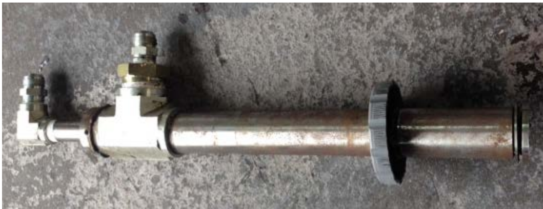
Figure 11 – “Mixer” nozzle design for aggressive mixing of grout/accelerant.
