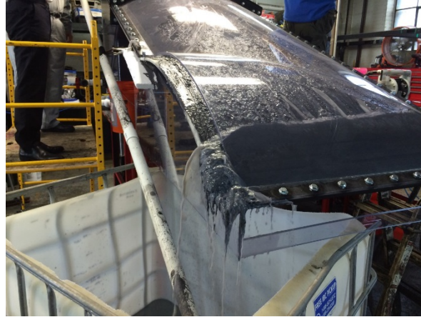
Figure 8 – U-gap results at 250 mm port.
