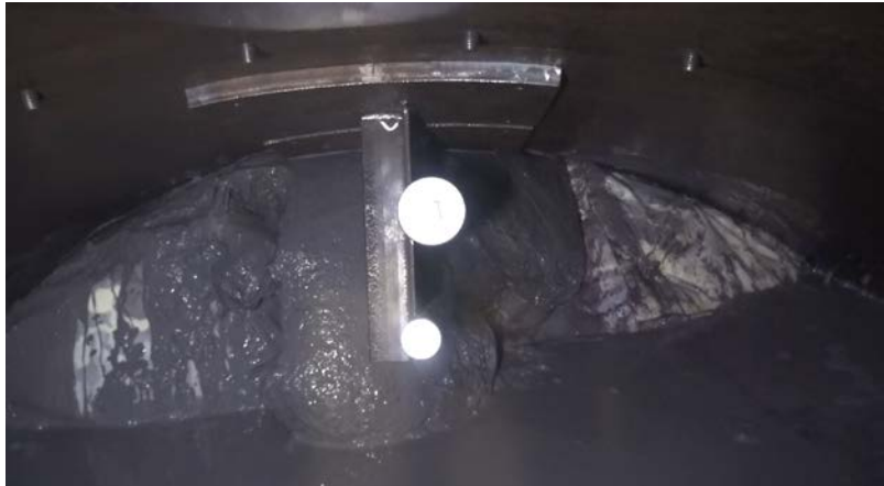
Figure 15 – V-gap plug as seen from gap entrance.
