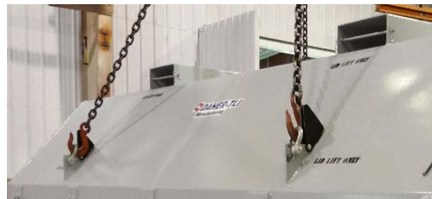
Upper subassembly lifted with lifting lugs
