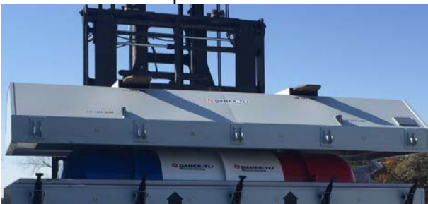
Upper subassembly lifted with fork pockets
